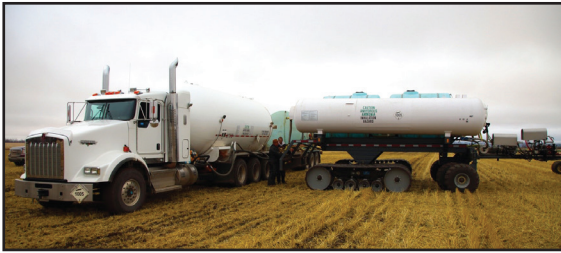
Pg. 10 - A Tridem field delivery truck and trailer at Manning, Alberta, Canada. At 8,000 gallons filling twin 2,000 gallon NH 3 tanks. The trailer is 5,000 gallons of liquid fertilizer, APP, ATS, KTS, Zn. Operating day and night applying 14,000 acres in October, 1,000 acres per day.
