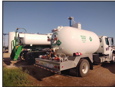
Pg. 16 - A 3,000 gallon delivery truck operating in a 60-mile radius filling the applicator every 3 hours in Nebraska conditions.
