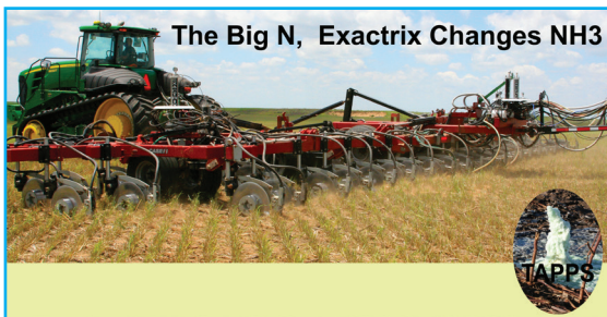
Pg. 15 - Mustang Tool Bar at 61.25 ft. 1 acre per minute at 8 mph. Banding deep @ 8" at Deerfield, KS.
