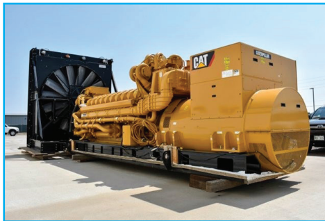
Cover - Caterpillar C-175-20 Diesel engine V-20 3,500 kw to 4,000 kw.
