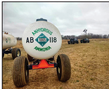
Pg. 14 - Nurse trailers will leave the agricultural scene. Like propane, NH3 liquid delivery is made to a high quality applicator, tank mounted or towed.
